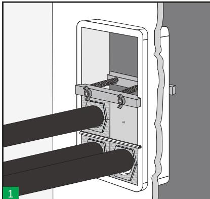
1 Clamp Tool can be used to fix blocks in their place when the transit installation is not completely finished.
