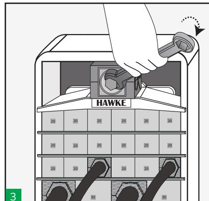
3 Once centred, we begin to tighten the compression tool which will be pressing on the compression plate.
