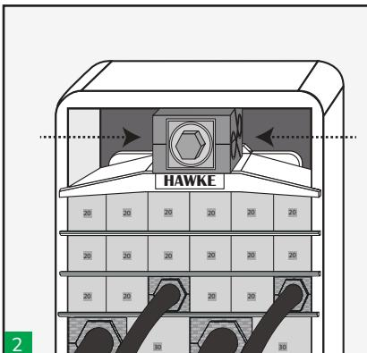
2 Compression tool must be introduced centred in the frame both in width and depth since otherwise the compression of the system would not be balanced so that to be able to introduce the lateral pieces of the endpacker it would be necessary to over tighten the tool and it could be damaged.
