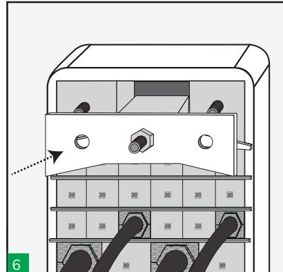
6 Insert the centre piece of the endpacker along with the front plate.
