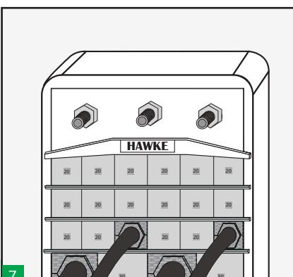
7 Tighten the nuts on the endpacker alternately following the above sequence to compress and complete the seal. Use a ratchet spanner for an easier installation. Approximately 10-12 mm of thread should protrude on each bolt to ensure the sealing.
