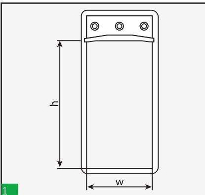
1 Before using the compression tool, it is important to check that the complete sealing area of this frame size (see table) is filled with blocks. Thus over tightening of the tool can be avoided.
