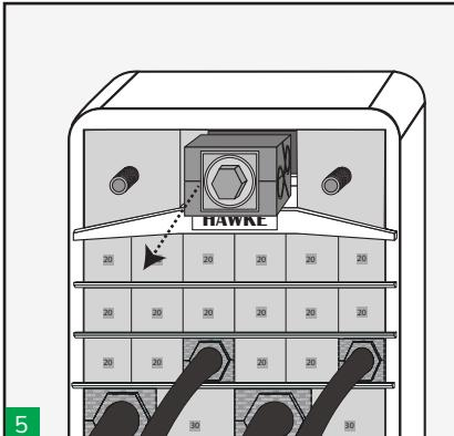
5 Insert the outer blocks of the endpacker. Then, untighten the compression tool and remove it.
