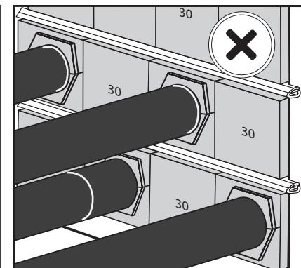
Check that marks in all the cables are visible to be guarantee blocks and cable copper tapes are aligned.
