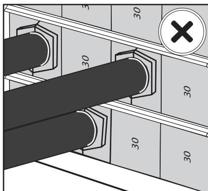
Check the correct orientation of the blocks.
