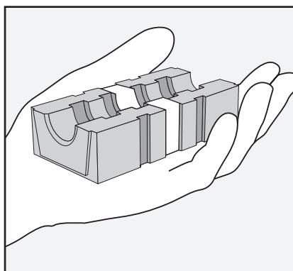
Measure the outer diameter of the cable and ensure that the diameter is within the cable range marked on the front of the block.
