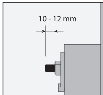
Check that the right tightening of the bolts have been performed (approximately 10-12 mm of thread on each bolt should protrude from the nut).
