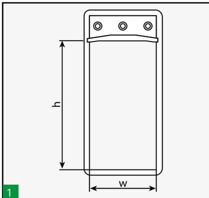
Before using the compression tool, it is important to check that the complete sealing area of this frame size (see table) is filled with blocks. Thus over tightening of the tool can be avoided.
