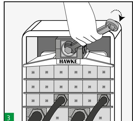
Once centered, we begin to tighten the compression tool which will be pressing on the compression plate.
