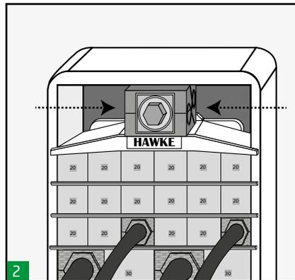
Compression tool must be introduced centered in the frame both in width and depth since otherwise the compression of the system would not be balanced so that to be able to introduce the lateral pieces of the endpacker it would be necessary to over tighten the tool and it could be damaged.
