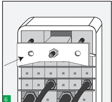
6 Insert the centre piece of the endpacker along with the front plate.
