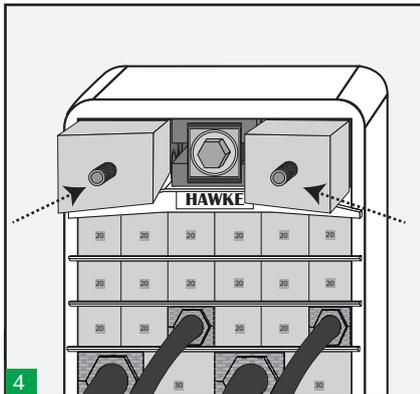
4 Before reaching the limit of tightening we must check if we have enough space to introduce the endpacker lateral pieces to avoid over tightening the tool that could block it.
