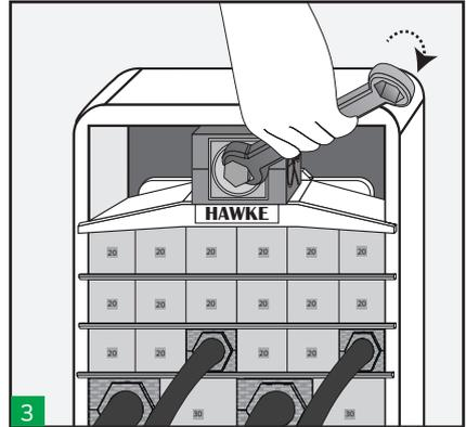
3 Once centred, we begin to tighten the compression tool which will be pressing on the compression plate.
