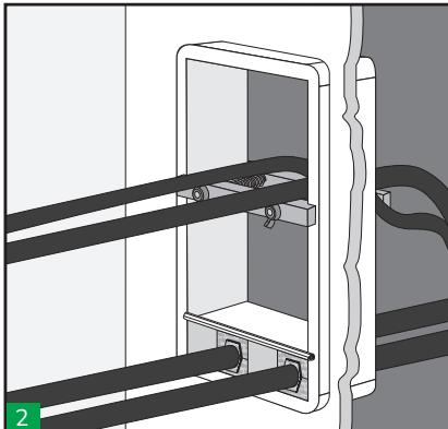
2 Clamp tool can be used to fix cables on the top part of the penetration allowing an easier installation of blocks.
