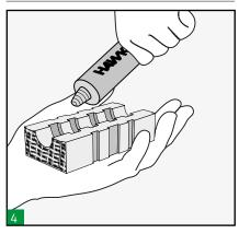
Lubricate all the insert and blank blocks using Hawke lubricant.
