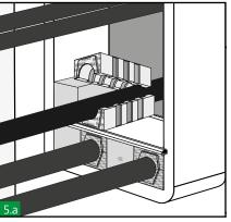
Begin packing the frame. Colour code will help you to install the blocks correctly. A stayplate is always inserted between each layer of blocks. Blocks should not protrude out of the stayplates retaining lips.
