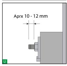
Approximately 10-12 mm of thread should protrude on each bolt to ensure the sealing.
