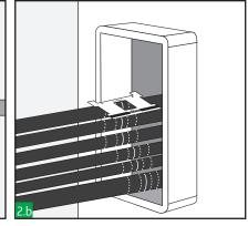
Mark each cable in the centre of the frame and 7-8mm either side of this point. Also, recommendable to mark the cable in both ends of the frame. EMC marking tool could help you to reduce time and ensure a correct marking.
