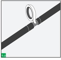
Using copper tape provided tightly wrap around the exposed screen until the cable outer diameter is regained.
