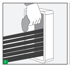
Make sure the frame is clean, then pull cables or pipes through, placing the largest at the bottom. (Note: Use open ended frame to fit around existing cables/pipes)
