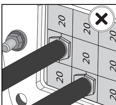
Check the correct orientation of the blocks.
