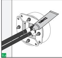
Lubricate the inside of the HRTO and all the insert and blank blocks using Hawke lubricant. Be careful don't contaminate the copper tape.
