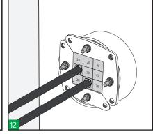
Tighten the nuts approximately 2mm each time following alternate tightening sequence, applying equal pressure to both plates.
