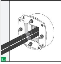
Cut and remove cable sheath between two central marks, to expose the cables conductive screen.
