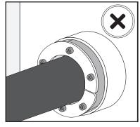
Check that the HRST is completely inserted in the Sleeve/Aperture.
