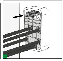
Pack the last row between the last stayplate and the compression plate. Insert the compression tool on the top, in the centre of the compression plate.
