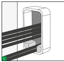
Insert HF200/R20 or HF300/ R20 round corner blocks in the bottom corners of the frame.
