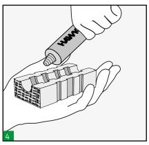
Lubricate all the insert and blank blocks using Hawke lubricant.
