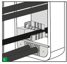
Begin packing the frame. Colour code will help you to install the blocks correctly.
