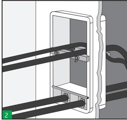
Clamp tool can be used to fix cables on the top part of the penetration allowing an easier installation of blocks.
