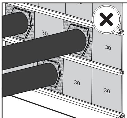
Check that there are a stayplate between each row of blocks and there are not stayplate between the bottom row of blocks and the frame.
