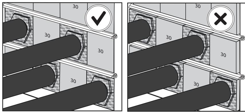
Check that HTS Lubricant has been used during the installation.
