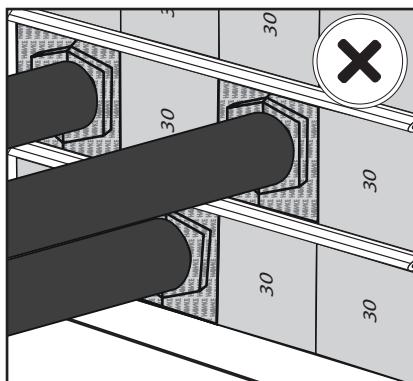
Check the correct orientation of the blocks.
