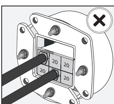
Check that stayplates have not be used in the installation.
