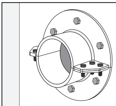
Check that HTS Sleeve has been used in the installation, that it has been properly installed (welded/bolted) and that it has not mechanical or corrosion damage.
