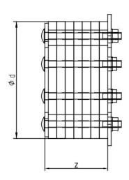
$\emptyset$ A-d depends on corrugated tube internal diameter.  $\square$ W depends on cables' quantity and size.
