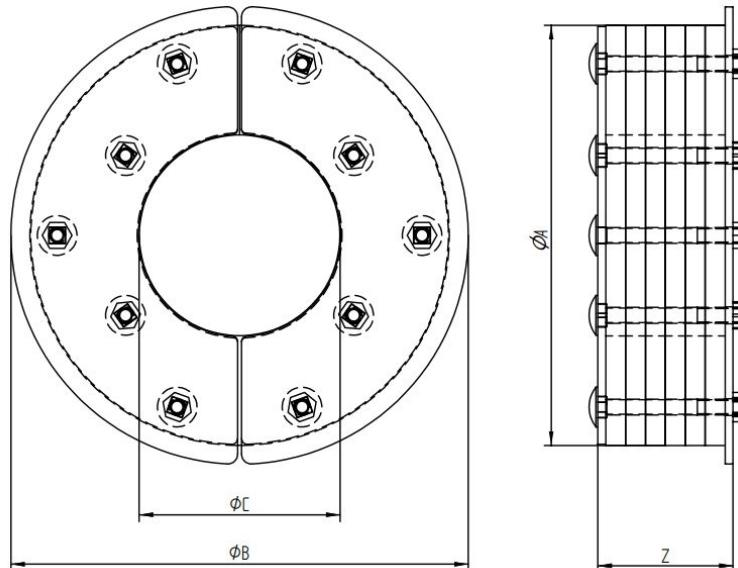
ØA-B depends on corrugated tube internal diameter.
