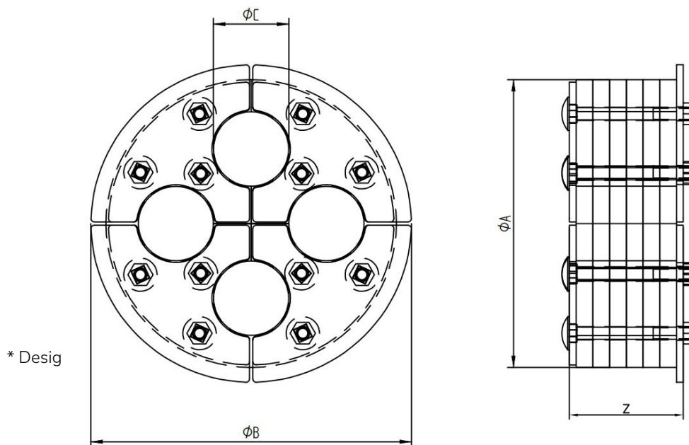
$\emptyset A$ - $B$  depends on corrugated tube internal diameter.
