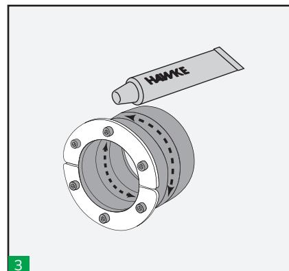
3 Lubricate the inside of the HRST to be in contact with the cable/ pipe and lightly lubricate the outside in contact with the sleeve.
