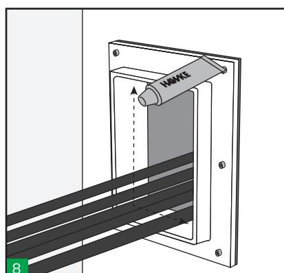
8 Lubricate the inside of the frame. Make sure the corners are well lubricated.
