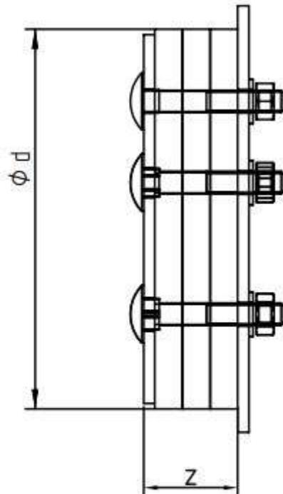
$\text{ØA-d}$  depends on corrugated tube internal diameter
