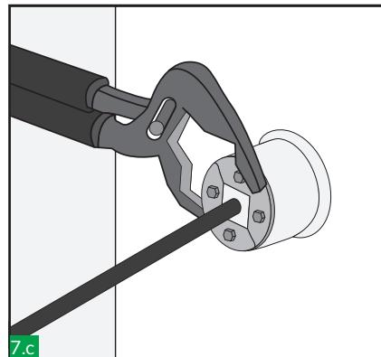
Slide the two front plates together and keep it fixed. Ensure all the blocks are located inside the front retaining lip.
