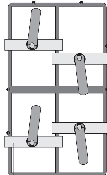
■ Welding tool (See page..80) can be used to prevent deformation during the welding.
