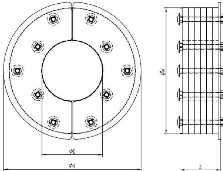
ØA-B depends on corrugated tube internal diameter.
