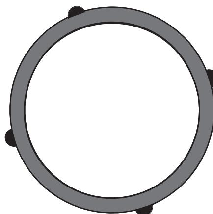
3. Start welding the frame with a sealing fillet weld on the backside. Follow appropriate welding sequence. This welding throat should not exceed of 3mm.
