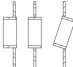
2. Tack weld on the front side, centring the frame onto the cut-out hole:
