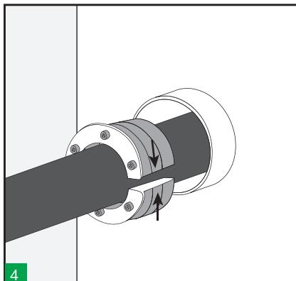
4 Open the HRST and install around the cable/pipe.
