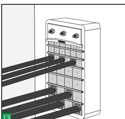
Make a visual inspection of the transit. HTS's unique colour coding system enables the installation to be visually inspected after completion and ensures correct matching of the block halves.
