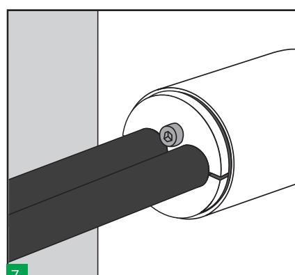
7 Make a visual inspection of the transit. HRST selected match the cables and sleeve installed, HRST is completely inserted into the sleeve, does not exist gaps between HRST and the cable/pipe.
