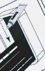
Lubricate the inside of the frame
