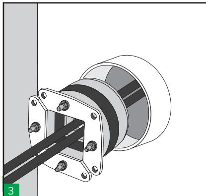
3 Insert the round transit frame completely in the sleeve/aperture around the cables. No lubricant should be applied to the aperture or outside of the frame. If close version of the Round Transit(HRT) is used, it should be installed previously to pull the cables/pipes through the sleeve or aperture.
