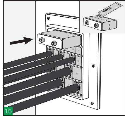
15 Pack the last row between the two last stayplates. Lubricate and insert H-DM endpacker at the top of the frame.
