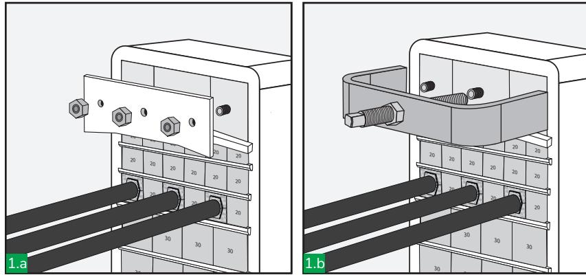
Remove endpacker nuts and front plate.
