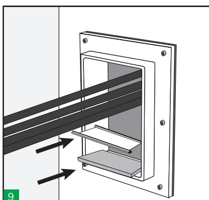
9 Before starting the sealing, place a 5mm strip with a stayplate at the bottom of the frame. These are included with compression system.
