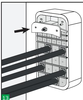
13 Insert the centre piece of the endpacker along with the front plate.
