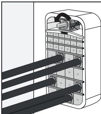
10 Tighten the compression tool until there is sufficient room to fit the outer blocks of the endpacker.
