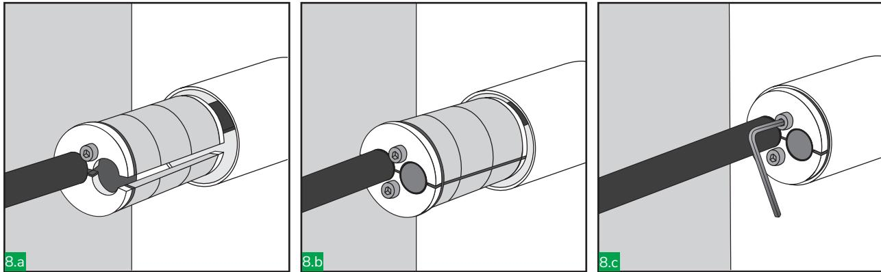
In case of any HRST hole are not occupied by cables always complete with HTS HRST plugs.
