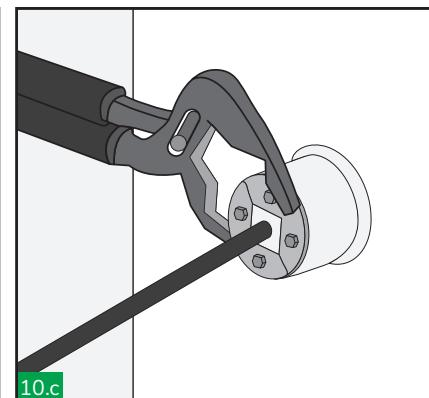
Slide the two front plates together and keep it fixed. Ensure all the blocks are located inside the front retaining lip.
