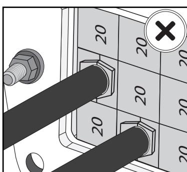
Check the correct orientation of the blocks.
