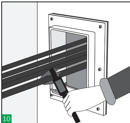
10 Take measures of the cables diameter with a calibre and select the appropriate HTS tolerant blocks. Colour code will help you to select the correct ones.
