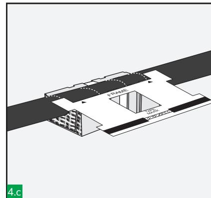
EMC marking tool could help you to reduce time and ensure a correct marking.
