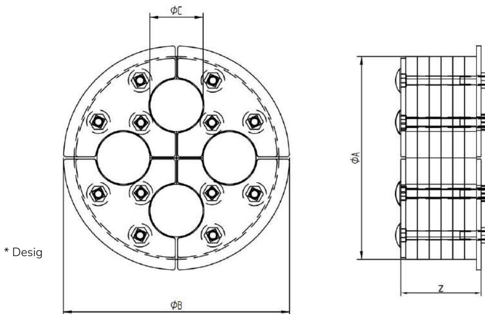
ØA-B depends on corrugated tube internal diameter.
