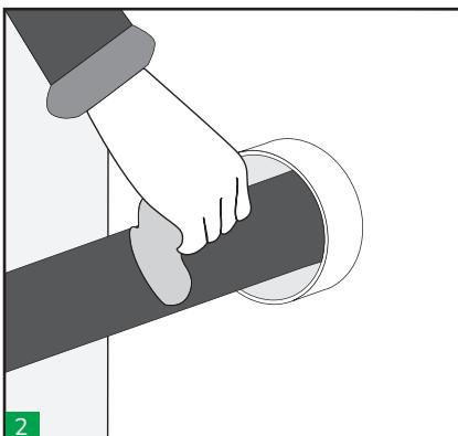
2 Make sure the pipe is properly centred in the sleeve. Make sure the sleeve and the cable/pipe are clean.
