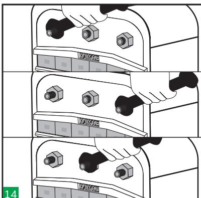
14 Tighten the nuts on the endpacking alternately following the above sequence to compress and complete the seal. Use a ratchet spanner for an easier installation.
