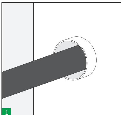
1 Check the inside diameter of the sleeve and the outside diameter of the cable/pipe to verify that it is within the range of selected HRST. HTS HRST colour code will help for a correct selection.
