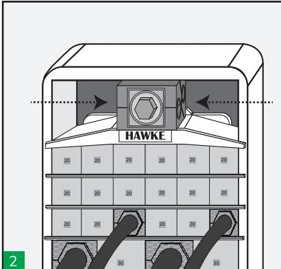
Compression tool must be introduced centred in the frame both in width and depth since otherwise the compression of the system would not be balanced so that to be able to introduce the lateral pieces of the endpacker it would be necessary to over tighten the tool and it could be damaged.
