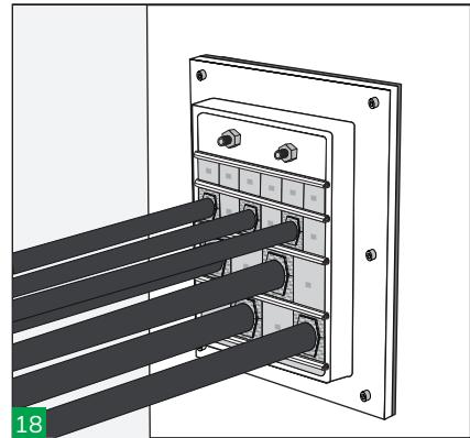
18 Make a visual inspection of the transit. HTS's colour coding enables the installation to be visually inspected after completion and ensures correct matching of the blocks halves.
