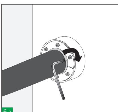
6.a Tighten the bolts. Tightening must be done in one revolution step for each bolt following next sequence until the system is enough compressed to seal the cable/pipe.
