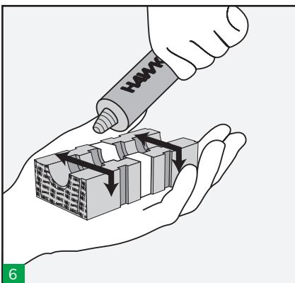
Very slightly lubricate all the insert and blank blocks using HTS lubricant taking care not to contaminate the copper on blocks and cables.
