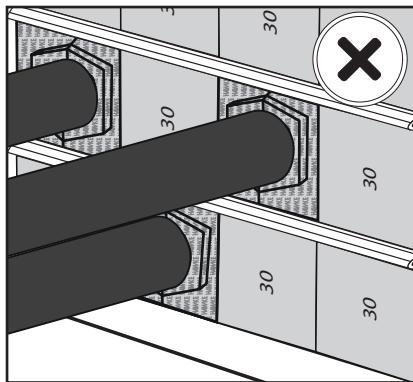
Check the correct orientation of the blocks.
