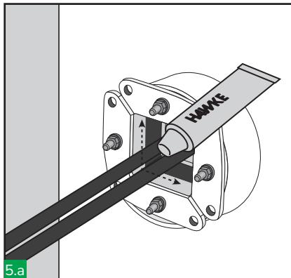
5.a Lubricate the inside of the HRTO and all the insert and blank blocks using HTS lubricant. Open the two front plates. (HRTO30, HRTO40 & HRTO50 front plates are fixed)
