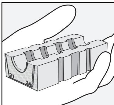
Measure the outer diameter of the cable and ensure that diameter is within the cable/pipe range marked on the front of the block or by the colour code of the block.
