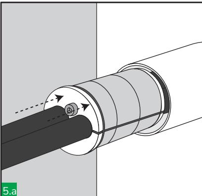
5.a Insert the HRST into the sleeve.
