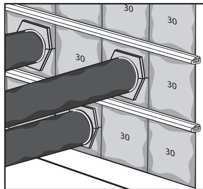
Check that HTS Lubricant has been used during the installation.
