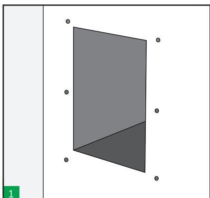
1 Cut a rectangular opening for the frame according to H-DH frame size to be used.(See table).
