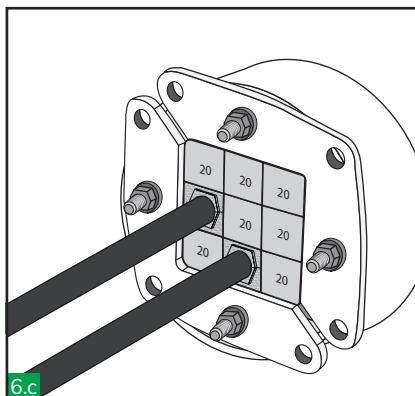
6.b 6.c Begin packing the transit frame starting at the bottom and finishing at the top. Ensure that the blocks are pushed firmly against the rear retaining lip. Verify that the complete sealing area of this frame size (see table) is filled with blocks.
