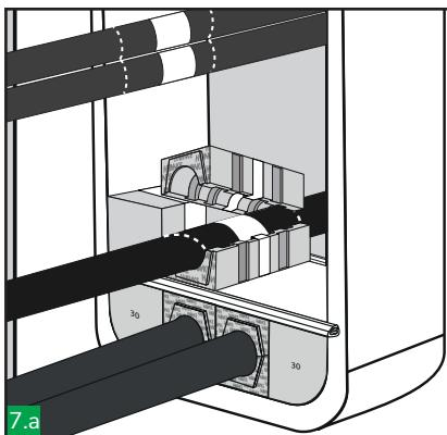
Begin packing the frame from the bottom to the top. A stayplate is always inserted between each layer of blocks. Blocks should not protrude out of the stayplates retaining lips. Ensure when fitting cables into blocks that copper tape on blocks and cable align. Marks in the cable will help to guarantee it.
