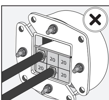
Check that stayplates have not been used in the installation.
