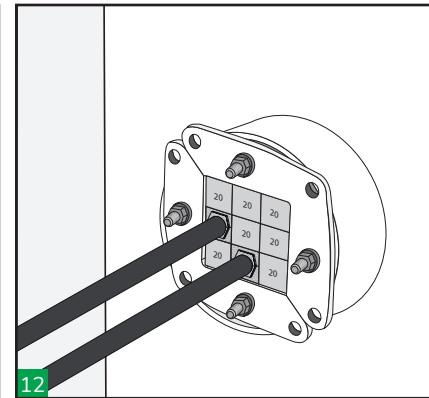
Tighten the nuts approximately 2mm each time following alternate tightening sequence, applying equal pressure to both plates. A minimum of 10 mm of thread should protrude on each bolt. Use a ratchet spanner for an easier installation.
