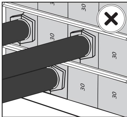
Check the correct orientation of the blocks.
