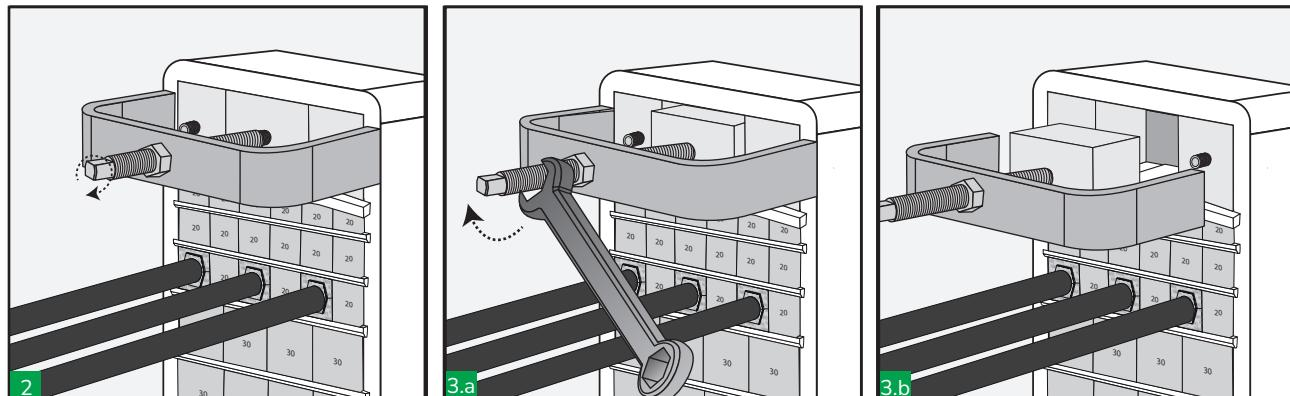
Turn the puller screw clockwise until it is fully screwed into the central piece of the endpacker.
