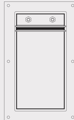
◆ Option 1 (recommended): Endpacker and stayplate located in upper end of the frame. Dm50 compensation module located on the bottom end, with a stayplate over it (never between module and frame).
