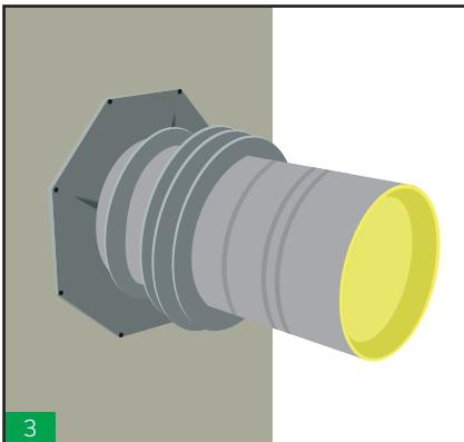
The wall sleeve is now installed and the wall formwork can be closed.
