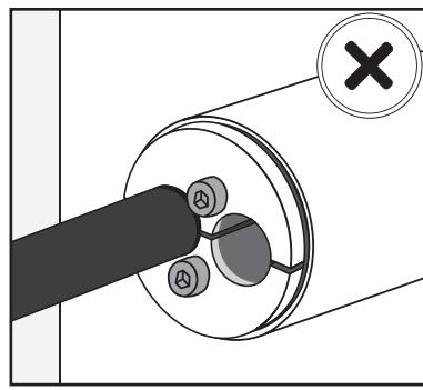
Check that every not occupied HRST holes are plugged with HTS HRST plugs.
