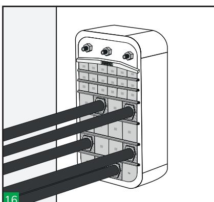
16 Make a visual inspection of the transit. HTS's unique colour coding system enables the installation to be visually inspected after completion and ensures correct matching of the block halves.
