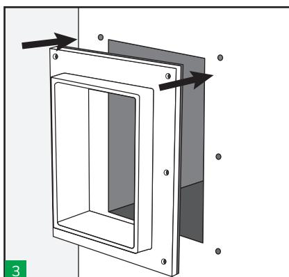
3 Install the frame in the opening with the gasket side towards the enclosure.
