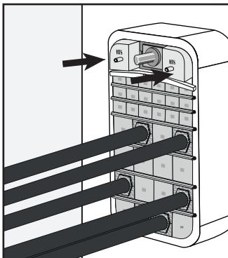
11 Insert the outer blocks of the endpacker. Then, untighten the compression tool and remove it.
