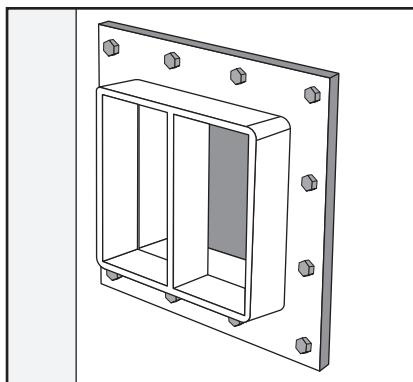
Check that HTS Frame has been used in the installation, that it has been properly installed (welded/bolted) and that it has not mechanical or corrosion damage.
