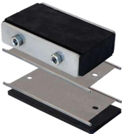
HTS CSDM Compression system is used in H-DM frames to compress and seal the installation of cables and DM modules. It includes the endpacker unit, 5mm filler strip and two stayplates. The 5mm filler strip can be installed as either the top or bottom row of blocks within a H-DM aperture.
