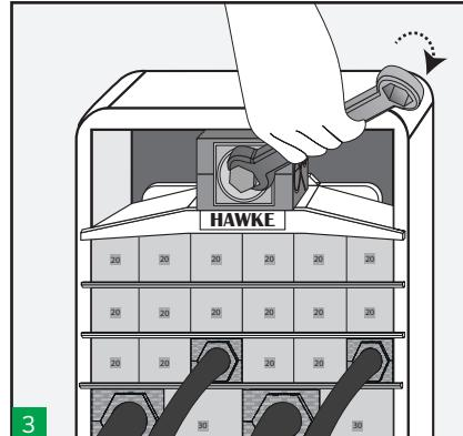
Once centred, we begin to tighten the compression tool which will be pressing on the compression plate.
