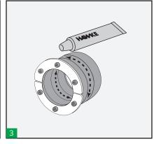
Lubricate the inside of the HRST to be in contact with the cable/ pipe and lightly lubricate the outside in contact with the sleeve.
