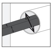
Check that the HRST is completely inserted in the Sleeve/Aperture.
