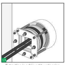
Extraction is achieved by releasing the compression, i.e. by reversing steps 10 and 11 and screwing M8 bolts (not supplied) into the threaded holes at each corner of the front plates. These releases the assembly from the aperture and allows the system to be disassembled.
