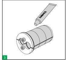
Lubricate the inside of the HRST to be in contact with the cables and lightly lubricate the outside in contact with the sleeve.
