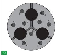
Tighten the screws incrementally, approximately 2 mm at a time, following the sequence shown in the pictured. Continue tightening until the system is fully compressed to seal the cable/pipe effectively.
