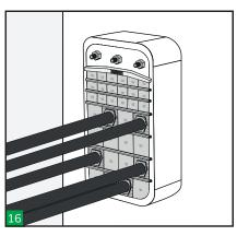
Make a visual inspection of the transit. HTS's unique colour coding system enables the installation to be visually inspected after completion and ensures correct matching of the block halves.
