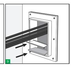
Before starting the sealing, place a 5mm strip with a stayplate at the bottom of the frame. These are included with compression system.
