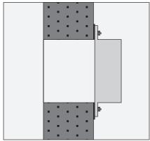
Size to fixing holes and type of fastener is to be established by the civil contractor dependent on size of sleeve weight and structure to which it is to be fixed. When fixing sleeves to concrete/brick type structure care should be taken if using expanding type fixings as they could burst into the aperture.
