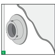
Tighten both pieces firmly. Use a hook wrench if necessary. Once tightened remnove excess of silicone.
