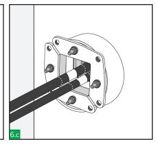
Using copper tape provided tightly wrap around the exposed screen until the cable outer diameter is regained. Repeat these steps for all cables.
