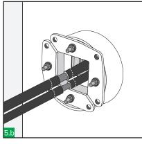
Cut and remove cable sheath between two central marks, to expose the cables conductive screen.
