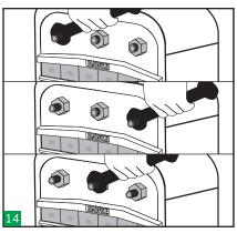
Tighten the nuts on the endpacking alternately following the above sequence to compress and complete the seal.
