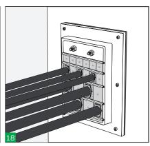
Make a visual inspection of the transit. HTS's colour coding enables the installation to be visually inspected after completion and ensures correct matching of the blocks halves.
