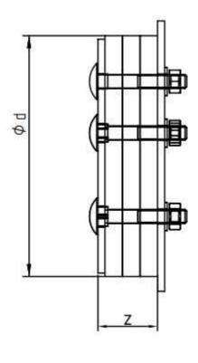
ØA-d depends on corrugated tube internal diameter
