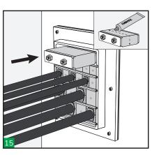
Pack the last row between the two last stayplates. Lubricate and insert H-DM endpacker at the top of the frame.
