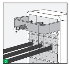
Turn the puller screw clockwise until it is fully screwed into the central piece of the endpacker.
