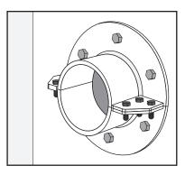
Check that HTS Sleeve has been used in the installation, that it has been properly installed (welded/ bolted) and that is has not mechanical or corrosion damage.
