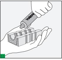
Lubricate all the insert and blank blocks, using HTS lubricant.
