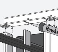
If HCOX open frame is used, Mastic/Silicone should be applied also in all bolting areas of the removable end as showed below.
