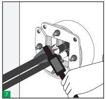
Take measures of the cables diameters and select the appropriate HTS Tolerant Blocks.
