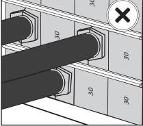
Check the correct orientation of the blocks.
