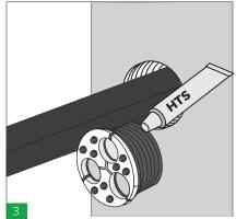
Lubricate the inside of the HBRST where it contacts the cable, and lightly lubricate the outside where it contacts the tube.
