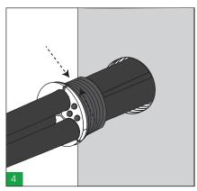
Open the HBRST and install it around the cable(s).
