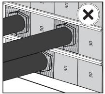
Check the correct orientation of the blocks.
