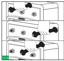
Tighten the nuts on the endpacking alternately following the above sequence to compress and complete the seal.
