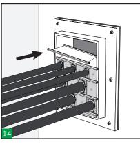
Insert the last stayplate before the last row of blocks (or earlier if required). Verify that the complete sealing area of this frame size (see table) will be filled with blocks. Note: 5mm strip supplied with the
