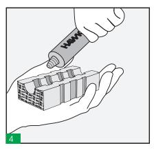
Lubricate all the insert and blank blocks using HTS lubricant.
