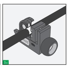
EMC cable sheath remove tool could help you to reduce time and ensure a correct cutting.
