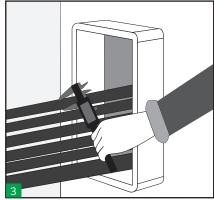
Take measures of the cables diameters and select the appropriate HTS Tolerant blocks. Colour code will help you to select the correct ones.
