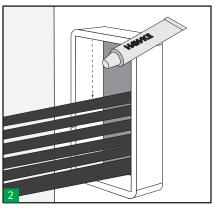
Lubricate the inside of the frame. Ensure the corners are well lubricated.
