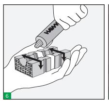
Very slightly lubricate all the insert and blank blocks using HTS lubricant taking care not contaminate the copper on blocks and cables.
