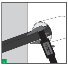
Check the inside diameter of the sleeve and the outside diameter of the cables to verify that it is within the range of selected HRST.
