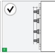
Conduct a final visual inspection of the installation, ensuring the following: The tightening has been uniform. The rubber seal fully embraces the cable and protrudes slightly through the front plate.
