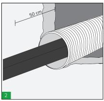
Confirm that cables enter the wall perpendicularly for at least 50 cm before reaching the tube.
