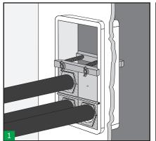
Clamp Tool can be used to fix blocks in their place when the transit installation is not completely finished.
