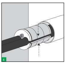
Open the HRST and install around the cables.
