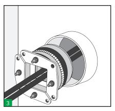
Insert the round transit frame completely in the sleeve around the cables and open the two front plates. (HRTO30,HRTO40&HRTO50 front plates are fixed). No lubricant should be applied to the aperture or outside of the frame.
