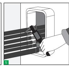
Take measures of cables diameters and select the appropriate HTS tolerant blocks.
