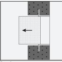
When all shuttering and other formwork has been removed, the polystyrene mould must be removed prior to electrical installation.
