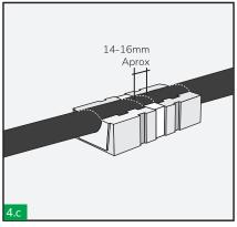
Mark each cable in the centre of the frame and 7-8mm either side of this point.
