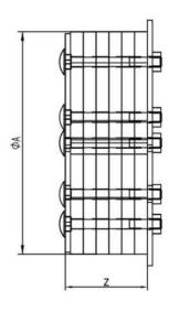
ØA-B depends on corrugated tube internal diameter. ØC depends on cables' size
