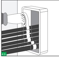
Using copper tape provided tightly wrap around the exposed screen until the cable outer diameter is regained.
