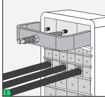
Remove endpacker nuts and front plate.
