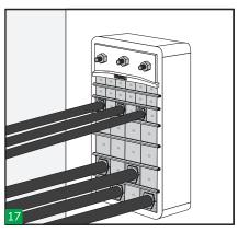
Make a visual inspection of the transit. Check that marks in all the cables are visible to be guarantee blocks and cable copper tapes are aligned.
