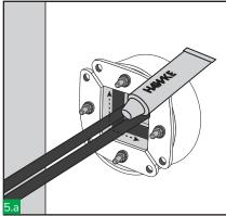
Lubricate the inside of the HRTO and all the insert and blank blocks using HTS lubricant. Open the two front plates. (HRTO30, HRTO40 & HRTO50 front plates are fixed)
