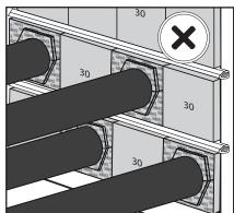
Check that HTS Lubricant has been used during the installation.
