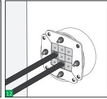
Tighten the nuts approximately 2mm each time following alternate tightening sequence, applying equal pressure to both plates.
