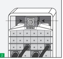
Compression tool must be introduced centred in the frame both in width and depth since otherwise the compression of the system would not be balanced so that to be able to introduce the lateral pieces of the endpacker t it would be necessary to over tighten the tool and it could be damaged.
