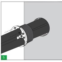
Carefully insert the HBRST into the tube. Ensure the HBRST is fully inserted so that the front plates are in direct contact with the tube.
