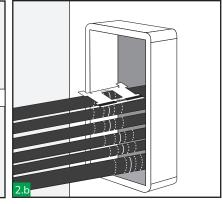
Mark each cable in the centre of the frame and 7-8mm either side of this point. Also, recommendable to mark the cable in both ends of the frame.
