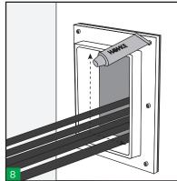
Lubricate the inside of the frame. Make sure the corners are well lubricated.
