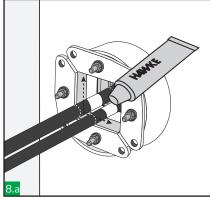
Lubricate the inside of the HRTO and all the insert and blank blocks using HTS lubricant. Be careful don't contaminate the copper tape.
