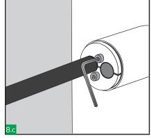
In case of any HRST hole are not occupied by cables always complete with HTS HRST plugs.
