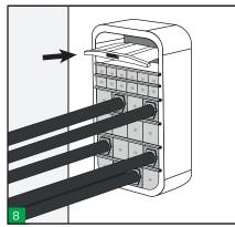
Insert the last stayplate and the compression plate before the last row of blocks (or earlier if required). Check frame packing space. Verify that the complete sealing area of this frame size (see table) will be filled with blocks.
