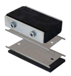
HTS CSDM Compression system is used in H-DM frames to compress and seal the installation of cables and DM modules. It includes the endpacker unit, 5mm filler strip and two stayplates. The 5mm filler strip can be installed as either the top or bottom row of blocks within a H-DM aperture.
