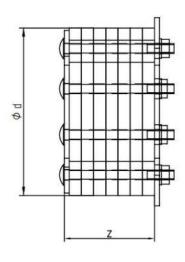
ØA-d depends on corrugated tube internal diameter.
