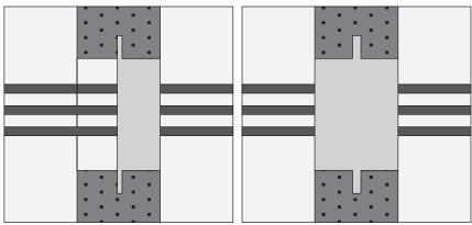
The sleeve can be casted directly into a wall or floor.
