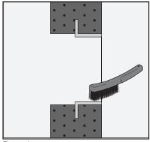
The transit aperture should be cleaned to remove any concrete or other debris that may have contaminated the apertures internal faces.
