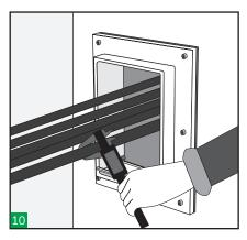
Take measures of the cables diameter with a calibre and select the appropriate HTS tolerant blocks. Colour code will help you to select the correct ones.
