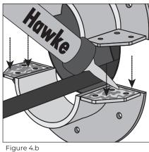
If CBO open sleeve is used, Mastic/Silicone should be applied also in all bolting areas of the removable end as showed below.
