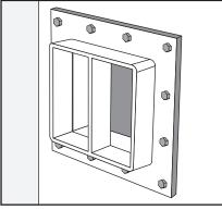
Check that HTS Frame has been used in the installation, that it has been properly installed (welded/bolted) and that it has not mechanical or corrosion damage.
