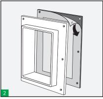
Remove the protection and stick the gasket on the aluminium frame.
