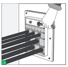
Tighten the nuts on the endpacker in alternate order to compress and complete the seal.
