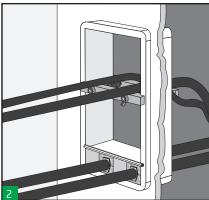
Clamp tool can be used to fix cables on the tope part of the penetration allowing an easier installation of blocks.
