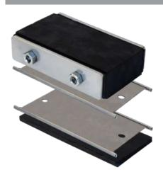
Hawke CSDM Compression system is used in H-DM frames to compress and seal the installation of cables and DM modules. It includes the endpacker unit, 5mm filler strip and two stayplates. The 5mm filler strip can be installed as either the top or bottom row of blocks within a H-DM aperture.
