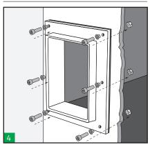
Insert bolts washers and nuts to the frame/ enclosure.
