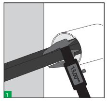
Check the inside diameter of the sleeve and the outside diameter of the cables to verify that it is within the range of selected HRST.
