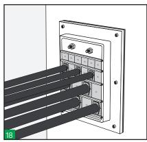
Make a visual inspection of the transit. Hawke's colour coding enables the installation to be visually inspected after completion and ensures correct matching of the blocks halves.
