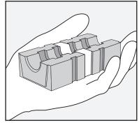
Measure the outer diameter of the cable and ensure that diameter is within the cable/pipe range marked on the front of the block.
