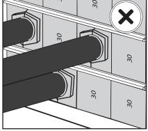
Check the correct orientation of the blocks.
