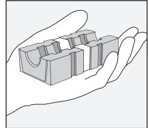
Measure the outer diameter of the cable and ensure that the diameter is within the cable range marked on the front of the block.
