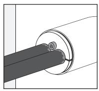
Check that all the bolts has been tightened similarly and do not exist gaps between the cable/pipe and the HRST.
