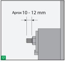
Approximately 10-12 mm of thread should protrude on each bolt.
