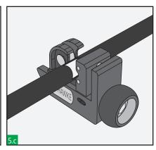
EMC cable sheath remove tool could help you to reduce time and ensure a correct cutting.
