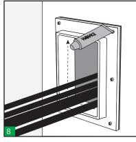
Lubricate the inside of the frame. Make sure the corners are well lubricated.
