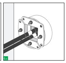
Using copper tape provided tightly wrap around the exposed screen until the cable outer diameter is regained. Repeat these steps for all cables.
