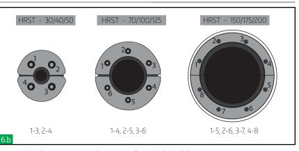
Tighten the bolts. Tightening must be done in one revolution step for each bolt following next sequence until the system is enough compressed to seal the cable/pipe.
