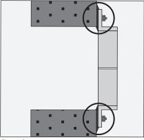
The frame can now be placed over its fixings and fasteners tightened to clamp the frame to the wall/floor.
