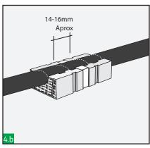
Mark each cable in the centre of the frame and 7-8mm either side of this point. Also, recommendable to mark the cable in both ends of the frame.
