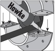
If CBO open sleeve is used, Mastic/Silicone should be applied also in all bolting areas of the removable end as showed below.
