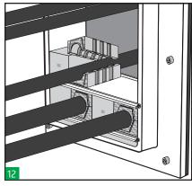
Keep sealing the transit from the bottom to the top using insert and blank blocks, as required.
