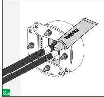
Lubricate the inside of the HRTO and all the insert and blank blocks using Hawke lubricant.
