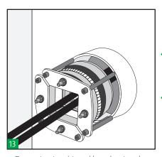
Extraction is achieved by releasing the compression, i.e. by reversing steps 10 and 11 and screwing M8 bolts (not supplied) into the threaded holes at each corner of the front plates. These releases the assembly from the aperture and allows the system to be disassembled.
