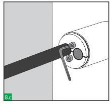
In case of any HRST hole are not occupied by cables always complete with Hawke HRST plugs.
