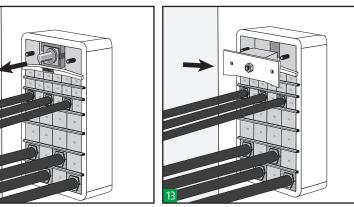
Insert the centre piece of the endpacker along with the front plate.
