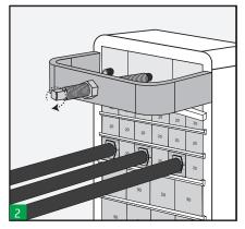
Remove endpacker nuts and front plate.
