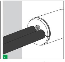
Make a visual inspection of the transit. HRST selected match the cables and sleeve installed, HRST is completely inserted into the sleeve, does not exist gaps between HRST and the cable/pipe.
