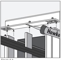
If HCOX open frame is used, Mastic/Silicone should be applied also in all bolting areas of the removable end as showed below.
