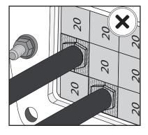
Check the correct orientation of the blocks.
