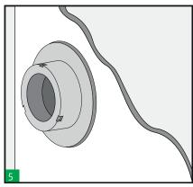
Tighten both pieces firmly. Use a hook wrench if necessary. Once tightened remnove excess of silicone.
