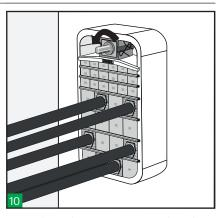
Tighten the compression tool until there is sufficient room to fit the outer blocks of the endpacker.
