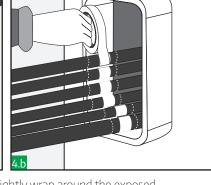
Using copper tape provided tightly wrap around the exposed screen until the cable outer diameter is regained.
