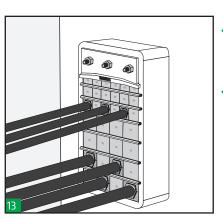
Make a visual inspection of the transit. Hawke's unique colour coding system enables the installation to be visually inspected after completion and ensures correct matching of the block halves.
