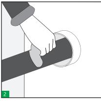
Make sure the pipe is properly centred in the sleeve. Make sure the sleeve and the cable/pipe are clean.
