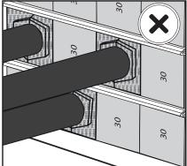
Check the correct orientation of the blocks.
