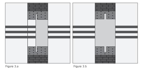
The sleeve may be cast into a concrete jacket. This method being normally used for brick and blockwork walls which in turn is fixed into the wall or floor.
