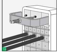
Remove endpacker nuts and front plate.
