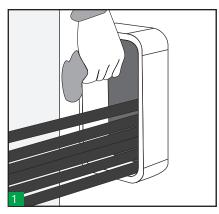
Make sure the frame is clean, then pull cables or pipes through, placing the largest at the bottom.
