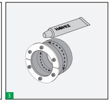
Lubricate the inside of the HRST to be in contact with the cable/ pipe and lightly lubricate the outside in contact with the sleeve.
