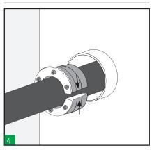
Open the HRST and install around the cable/pipe.
