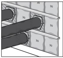
Check that there are sufficient blocks installed into the frame to cover the sealing area defined for each size of frame.
