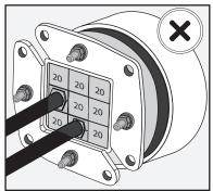
Check that the HRT/HRTO is completely inserted in the Sleeve/Aperture.
