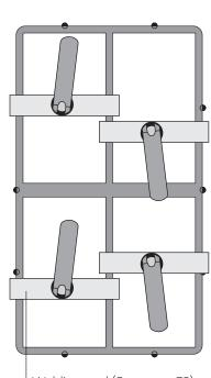
Welding tool (See page..78) can be used to prevent deformation during the welding.
