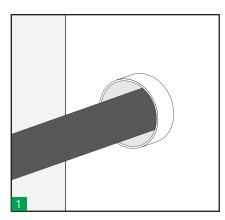
Check the inside diameter of the sleeve and the outside diameter of the cable/pipe to verify that it is within the range of selected HRST. Hawke HRST colour code will help for a correct selection.
