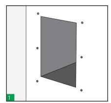
Cut a rectangular opening for the frame according to H-DH frame size to be used.(See table).
