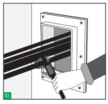
Take measures of the cables diameter with a calibre and select the appropriate Hawke tolerant blocks. Colour code will help you to select the correct ones.
