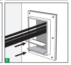
Before starting the sealing, place a 5mm strip with a stayplate at the bottom of the frame. These are included with compression system.
