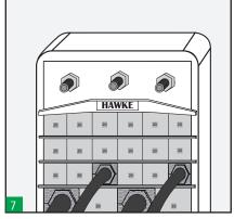
Tighten the nuts on the endpacker alternately following the above sequence to compress and complete the seal. Use a ratchet spanner for an easier installation. Approximately 10-12 mm of thread should protrude on each bolt to ensure the sealing.
