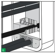
Begin packing the frame. Colour code will help you to install the blocks correctly.
