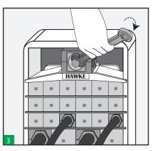
Once centred, we begin to tighten the compression tool which will be pressing on the compression plate.
