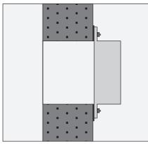
fastener is to be established by the civil contractor dependent on size of sleeve weight and structure to which it is to be fixed.
