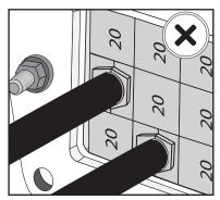
Check the correct orientation of the blocks.
