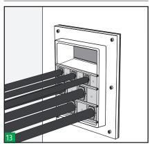
A stayplate is always inserted between each layer of blocks.
