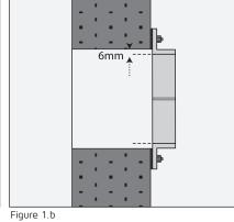
Size to fixing holes and type of fastener is to be established by the civil contractor dependent on size of frame weight and structure to which it is to be fixed. When fixing frames to concrete/brick type structure care should be taken if using expanding type fixings as they could burst into the aperture.
