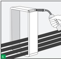
Final weld to form full radius at corners of frame.
