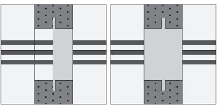
The sleeve can be casted directly into a wall or floor.
